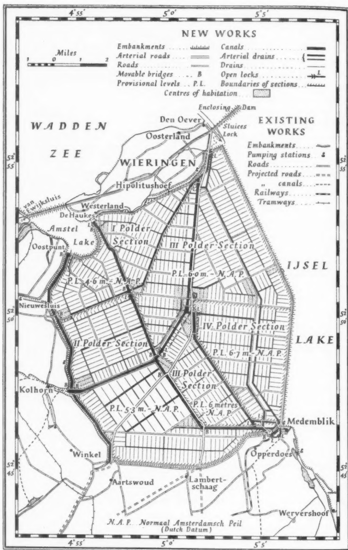
Fig. 6. The drainage scheme for the Wieringermeer polder
